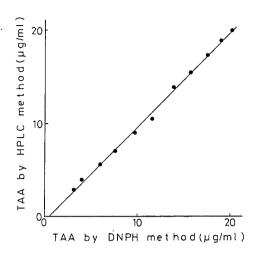
Fig. 3 Correlation between quantities of TAA estimated by DNPH method and by this HPLC method.
