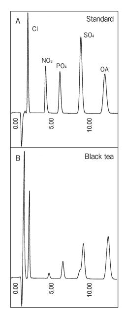
Fig. 1 Chromatograms illustrating the measurement of oxalic acid by ion chromatography.
