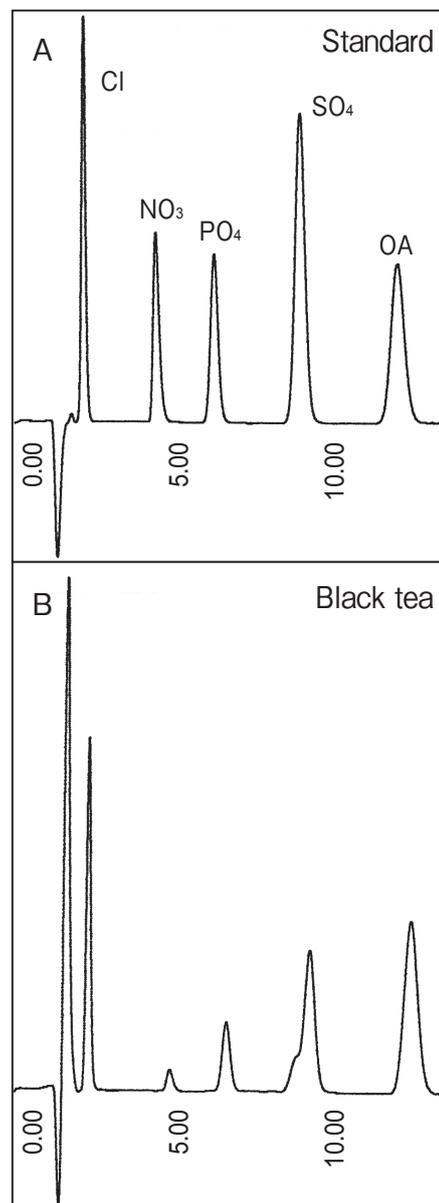
Fig. 1 Chromatograms illustrating the measurement of oxalic acid by ion chromatography.
